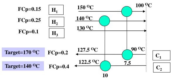
Assume the matches  $H_1$ - $C_1$  and the matches  $H_2$ - $C_2$  have been selected. Since  $H_3$  needs to go to the pinch temperature, there is no cold stream left to match, even if there is portions of  $C_1$  or  $C_2$  that are left for matching. Such matching would be infeasible.
