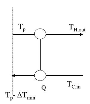
$$T_{C,in} = T_p - \Delta T_{min} - Q/FCp_C$$
