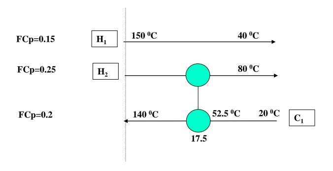
• The tick-off rule says that a maximum of 17.5 MW is exchanged in the match H2-C1 and as a result stream H2 reaches its target temperature.
