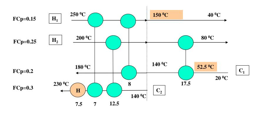
Below the pinch we try to have the cold streams start at their inlet temperatures and we later locate coolers (one in this case).
